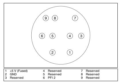
Figure 1-2. 9-Pin Mini-Circular DIN Connector
